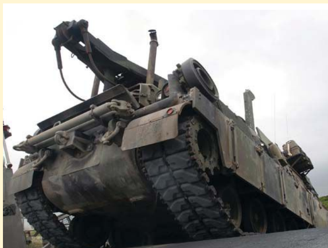
Figure 1 | A recent $108 million U.S. Army/BAE Systems contract covers the incarnation of 29 U.S. Army and 16 USMC M88A2 HERCULES recovery vehicles using remanufactured hulls. USMC photo by Lance Cpl. Jeremy T. Ross
